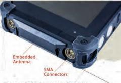
For an embedded antenna and two SMA connectors choose: WiFi, Bluetooth®, WWAN or GPS
