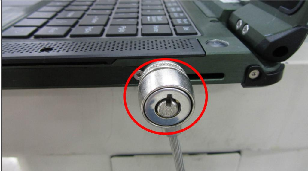
The Kensington lock slot is on the right side of the computer. Plug the Kensington lock into the slot and lock it. Both the computer and SSD are secured.
