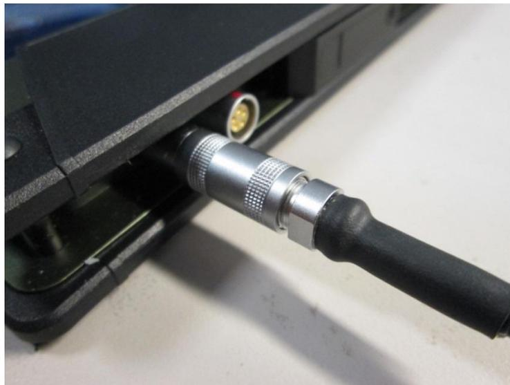
**Figure 3-1: Connecting the Flexpedient® AT80 Rugged Tablet to the Power Adapter**
