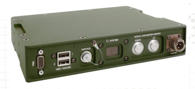
The KSW401 is a KVM switch for VGA and USB input in a fully rugged enclosure. It allows up to 7 computers to share the use of a single VGA and 2x USB for keyboard and mouse. You can also connect up to 3 KVM switches together, getting up to 19 computers on the same console. The peripheral focus will be given to a computer manually by using pushbuttons on the switch, or by commands on the keyboard.
