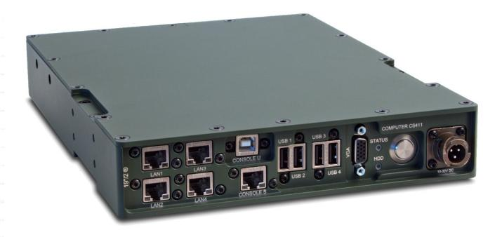
The 19"/2 Computer Atom CS401 is a rugged computer with the processing power of an Intel Atom D2550 1.86GHz processor in a compact, small form factor. The CS401 is optimized for size, weight (6.6 lbs), and low power consumption. Designed for rugged military applications in tough environments
