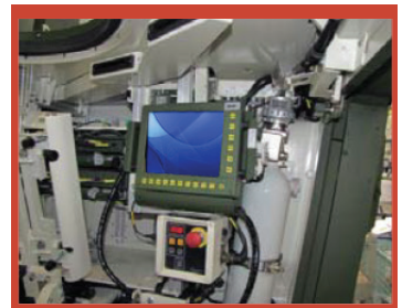
MOJAVE RD10 vehicle installation
