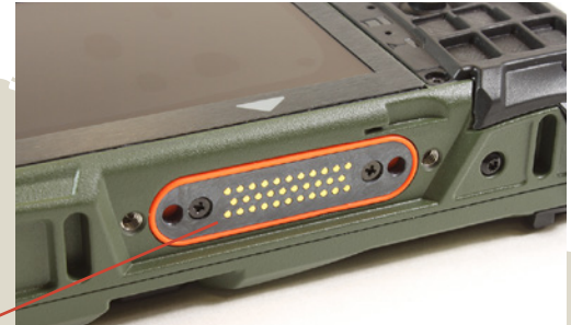
With plate off - Cradle POGO connector x 1
